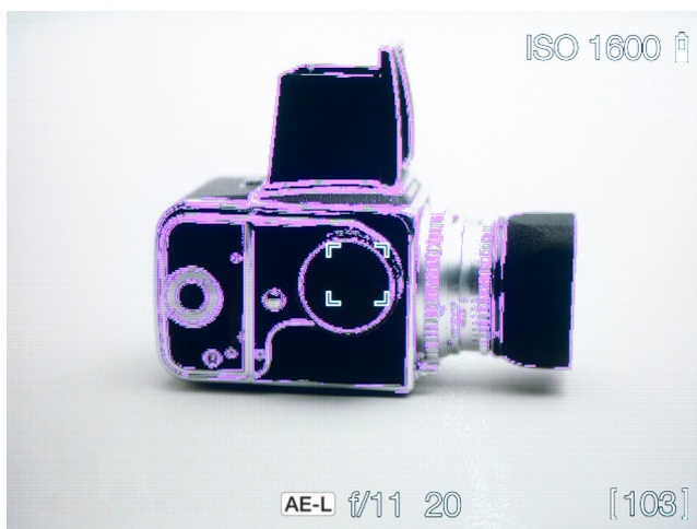
Focus Peaking display when subject parts are in focus
