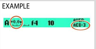
Viewfinder display indicating no adjustment to next frame and three frames left in the sequence.
