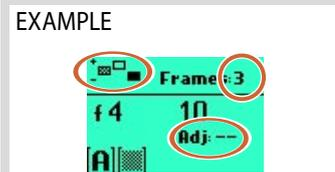
Screen after Bracketing setting activated indicating 3 frames remaining in a Standard, Over, Under, sequence with no adjustment to the next frame.
