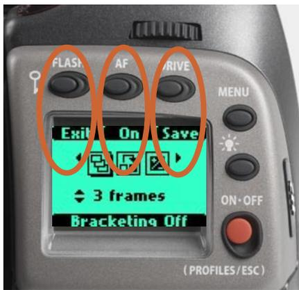
The basic principle behind making changes is that the appropriate button is first pressed to access the menu and then settings altered by way of the control wheels. The appropriate control wheel is designated by arrowheads alongside the setting description.
