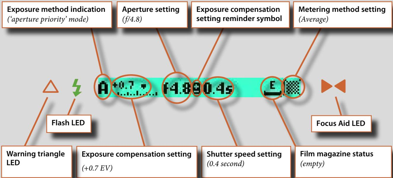
Some examples of various viewfinder LCD screens visible with standard settings and when specific control buttons are pressed.
