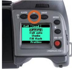
33. From the inactive mode, press the ON.OFF button until you see the H2 logo on the grip LCD. The LCD then in turn displays the 'main' screen. If the camera is already in 'standby' mode (the H2 logo will be visible on the grip LCD) click on either the shutter release button or the ON.OFF button to activate it again. (Note that a 'click' action is a quick press. See later section for a description of different button pressing actions)
